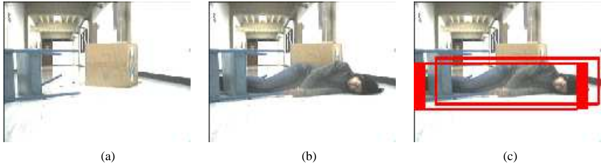
Fig. 5. Detecting a victim around office debris. (a) office debris, (b) victim occluded by the debris and (c) the system detecting the victim
